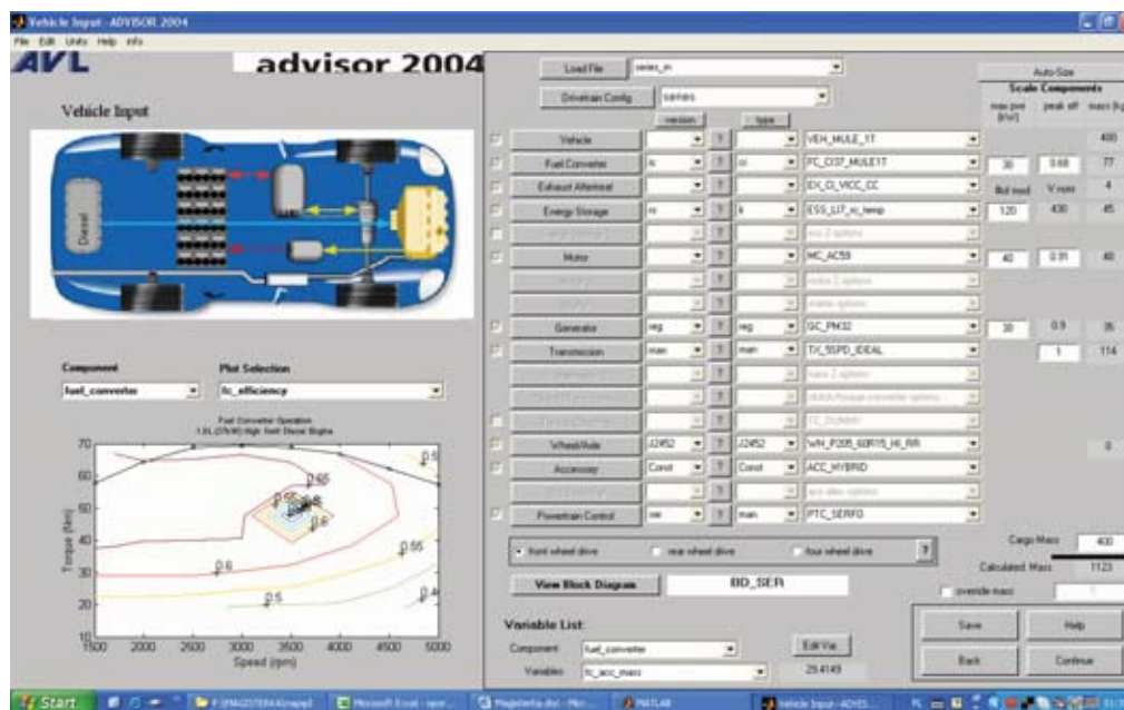
Rys. 4. Ekran interfejsu programu ADVISOR w wersji 2004 Fig. 4. Interface screen of the ADVISOR program version 2004
